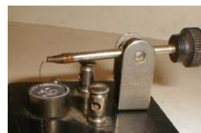
Figure 19.1: A galena crystal detector with cat's whisker.
